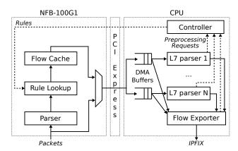
Fig. 2. Implemented 100 Gbps flow monitoring system
