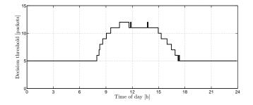
Fig. 5. Prototype deployment: value of heavy flow decision threshold
